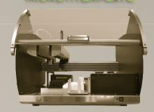
4 or 8 probes with robotic gripper on separate arms
