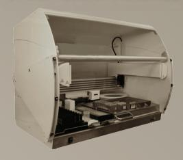
4 or 8 probes with robotic gripper on separate arms
